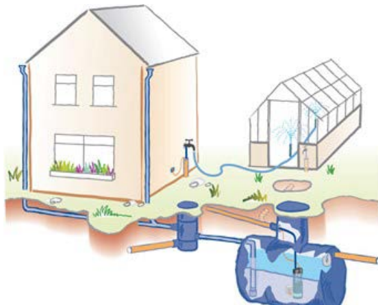
Fig. 3: Garden Rainwater Harvesting System
