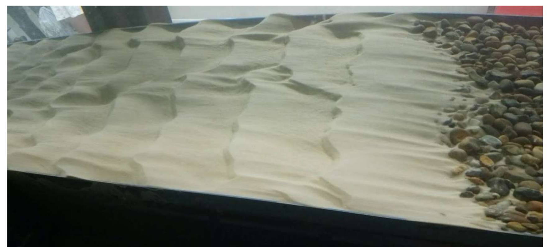
Experiment showing the formation of bedforms (sand dunes) in a flume
