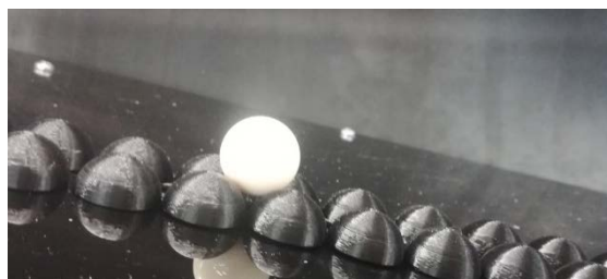
Fig. 4: The motion of a sphere rolling on top of other spheres (immersed in water) is tracked via a high-speed camera. This is used to obtain the added mass of the white sphere.
