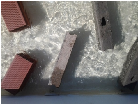
Fig. 4: Bricks used to create head drop
