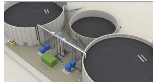
Fig. 6: PWS Biological Nutrient Removal process
