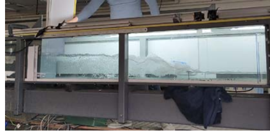
Fig. 6: Sudden deceleration experiment, Fr = 1.8
