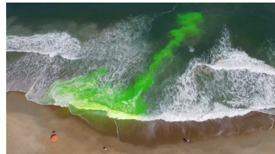
Fig. 4: Rip current, visualised with food dye
