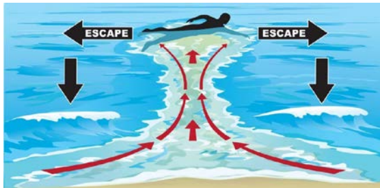
Fig. 5: Rip current mechanism
