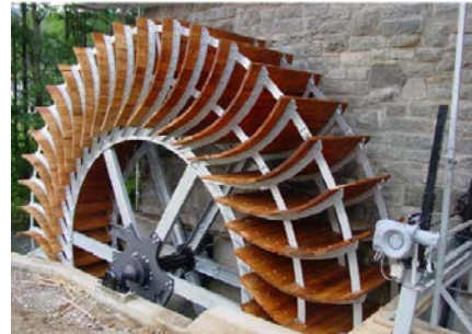
Fig. 2: Zuppinger low-head waterwheel
